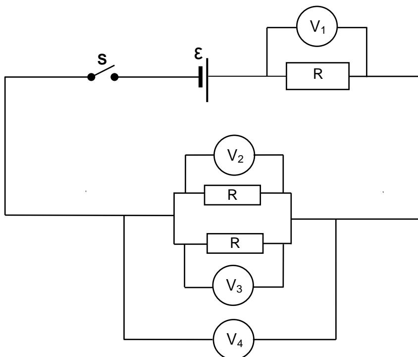
Which voltmeter will have the HIGHEST reading when switch **S** is closed?
