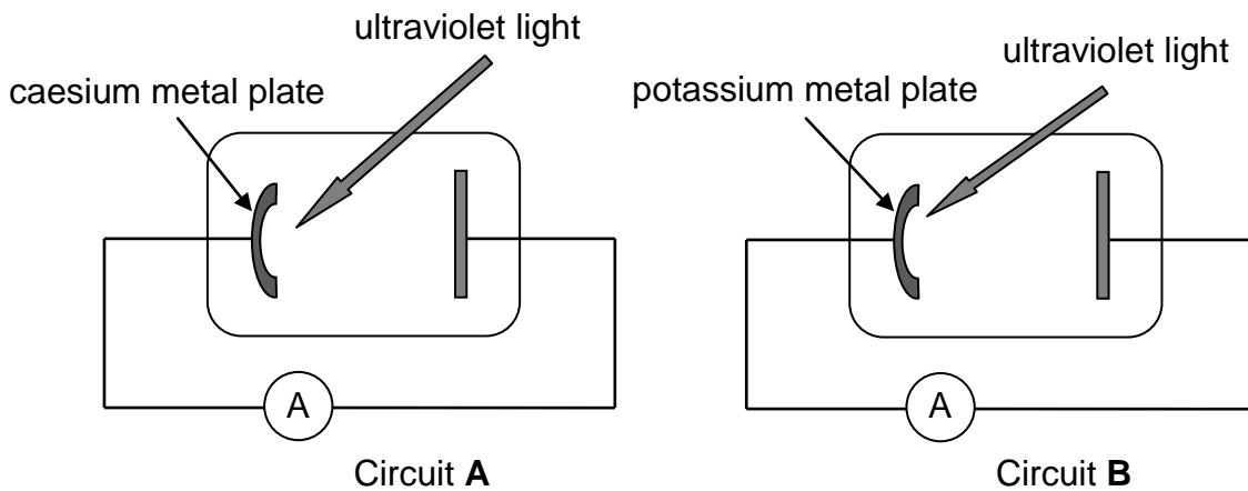
Ultraviolet light with the same intensity and wavelength of  $5,5 \times 10^{-7}$  m is incident on the metal plate in EACH of the photocells and the ammeter in circuit **A** registers a current.
