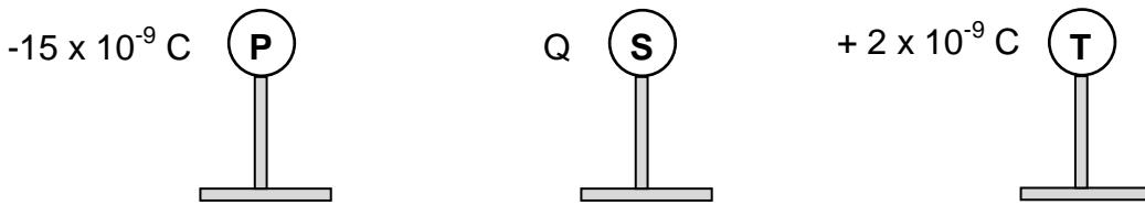
The charged spheres are brought together so that all three spheres touch each other at the same time, and are then separated. The charge on each sphere, after separation, is  $-3 \times 10^{-9}$  C.
