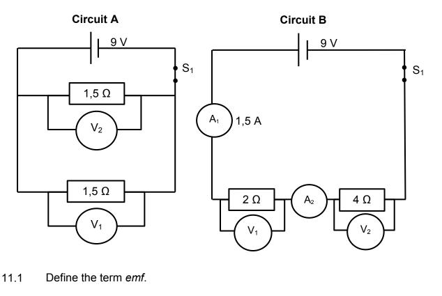
11.2 Calculate the total resistance of Circuit A.
