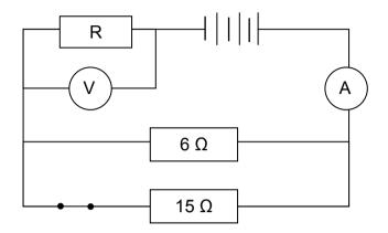
The total power dissipated in the parallel part of the circuit is 50 W.
